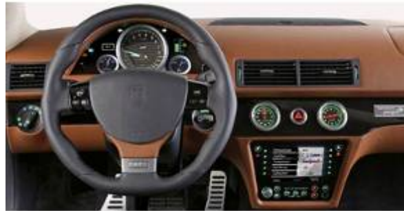
Artega - Artega GT (Dual-Dashboard Display) Fujitsu MB86R01 "Jade" graphics controller ARM926EJ-s + Jazelle Java Acceleration Technology
